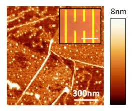
Fig. 1: (Colour on-line) Tapping mode atomic force microscope (AFM) image of a CVD graphene film transferred on  $SiO_2$ . Different thermal expansion of the Cu foil and the graphene sheet result in the formation of a few nm high ripples. Locally cracks can form during the transfer process and occasionally one is left with PMMA residues. Inset: Hall bar device used to measure the conductivity of CVD grown graphene (scale bar is  $5 \mu m$ ). Representative data is given in figs. 2 and 5.
